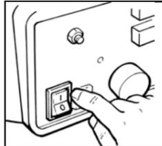
The priming cycle fills the boiler with water and flushes the system through. After this your Brewer will be ready for use.
