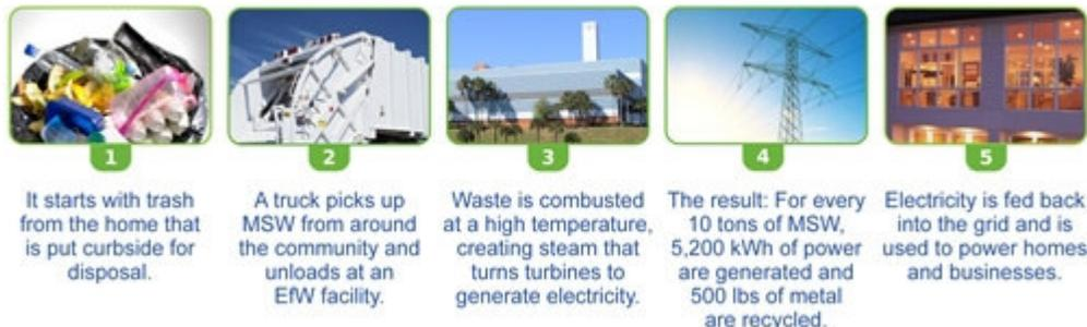
Energy-from-Waste (EfW) or waste-to-energy (WTE) is a process that takes municipal solid waste –including plain old household trash -- and transfers it into combustion chambers where it is reduced to 10% of its original volume in the process. The heat generated from the combustion chambers heats up water in steel tubes that form the walls of the combustion chambers. The water is turned to steam and sent through a turbine that continuously generates electricity.
